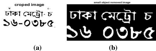
Fig 6: The left image is the extracted number plate image and the right one is dust removed image
